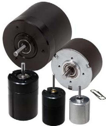
Figure 14: KinetiMax motors are outside-rotor BLDC motors with a high pole count (as many as 12) to minimize torque ripple. The outer-rotor design increases inertia for smoother running. With careful implementation, speed can be controlled to within 1% to 2% by the on-board electronic drive.
