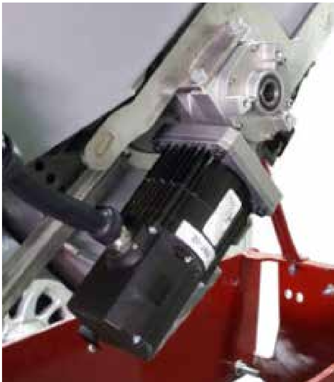
Gearmotors in the Graham Pro EPD incorporate a wireless control board embedded in the end cap of each motor, enabling each motor to communicate wirelessly.
