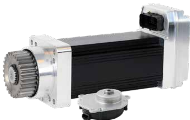
Figure 6: Allied Motion's EPS90 integrated steering motor actuator, shown with the SWS steering wheel sensor accessory, includes the motor, gearing, feedback sensor, and power and control electronics.
