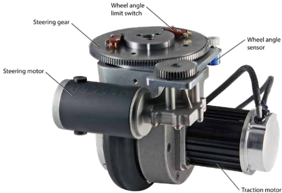
Figure 5: In this integrated traction-wheel assembly with steering package, the right-angle permanent-magnet gear motor turns a pinion that rotates the wheel about its centerline. The small white pinion and blue sensor provide feedback information to the vehicle controller to indicate the position of the wheel.
