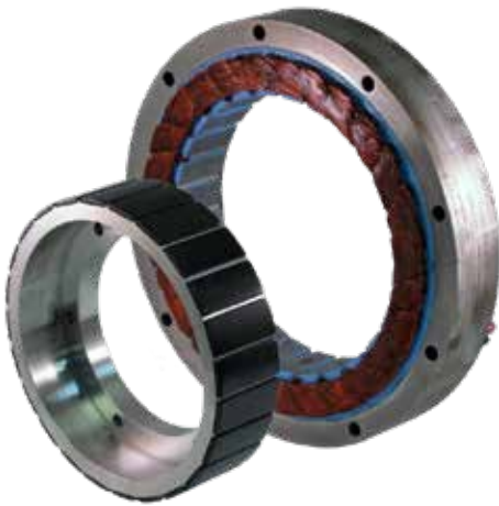
Figure 12: The stator (right) of a slotted BLDC torque motor features individual teeth around which the windings are placed. The example shown is a Megaflux frameless DC motor, which arrives as two separate elements that need to be built directly into the machinery. The picture also shows the individual magnet sections on the rotor (left). The outside diameter of the stator is 170 mm, and the width of the rotor is 25 mm.
