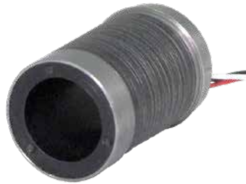
Figure 13: The stator of a PerformeX slotless motor, shown here without a housing, has no teeth to concentrate the windings. The lack of teeth eliminates cogging, leading to very smooth motion. The diameter of this stator is only about 20 mm. It is part of a motor used in high speed surgical handtools.
