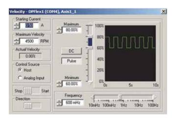
A built-in four-channel oscilloscope allows you to visually monitor results on the PC while adjusting tuning parameters. DP.D is capable of automatically determining the resistance and inductance of a motor to in order to set up current loop compensation. In addition, it will automatically determine the motor's start-up parameters.
