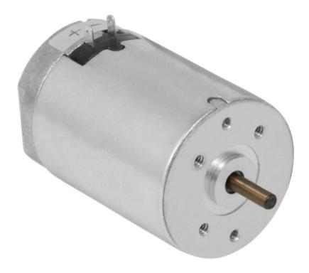
Allied Motion's IM-15 HP series motor is a 38.1 mm (1.5") brushed DC Permanent Magnet motor. Featuring strong and stable rare-earth Samarium Cobalt magnets, the IM-15 HP motor series delivers greater torque and high-pulse current without demagnetizing.
